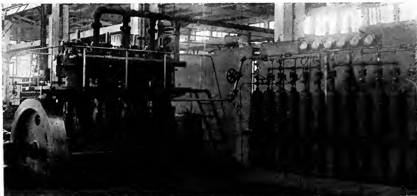
A Dow stationary Diesel on the test stand at the big Oakland plant of the Dow Pump and Diesel Engine Works.
